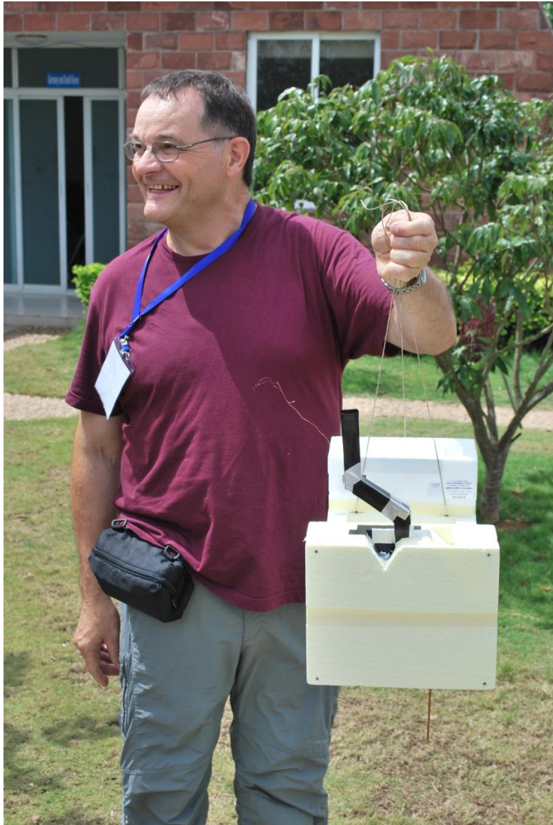
Meteolabor SRS-C34 radiosonde + Snow White chilled-mirror hygrometer
